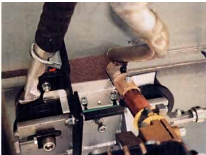
Close-up of the welding head.
