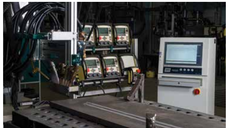
Multi-wire setup with PEK and WeldQAS
